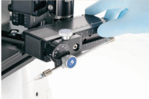
Swivel out function for easy capillary exchange.
